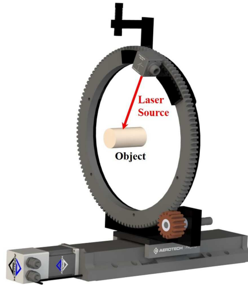
Figure 3-2. Light illumination using the source-positioning unit
