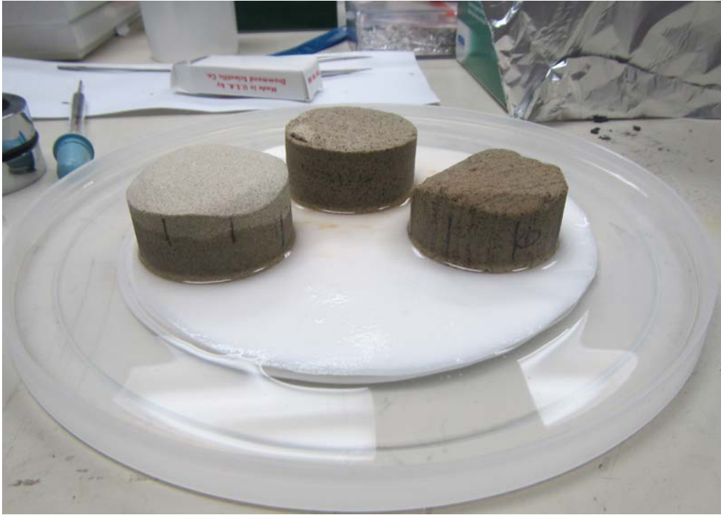
Fig. 6: Capillary Uptake: 20 min., Saturation of 1870 Stone
