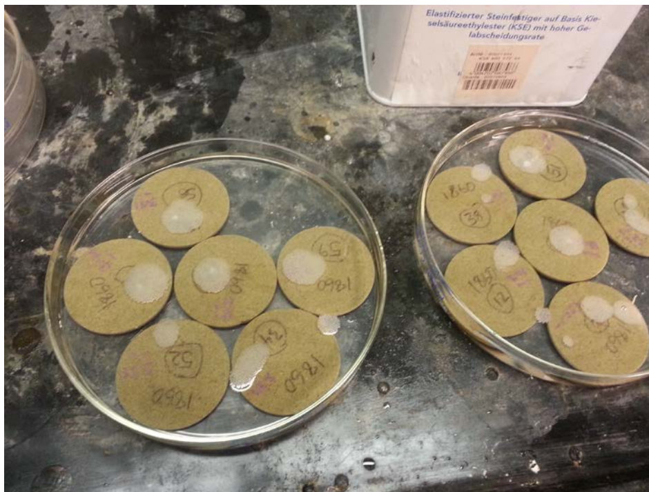
Fig. 18. During Testing Photo: Sample discs of stone submerged in consolidant. Photo by author.
