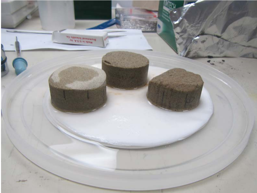
Fig. 8: Capillary Uptake: 40 min., Saturation of 1860 Stone
