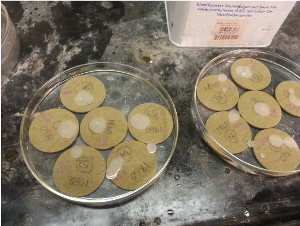
Fig. 21. During Testing Photo: Sample discs of stone submerged in consolidant. 94
