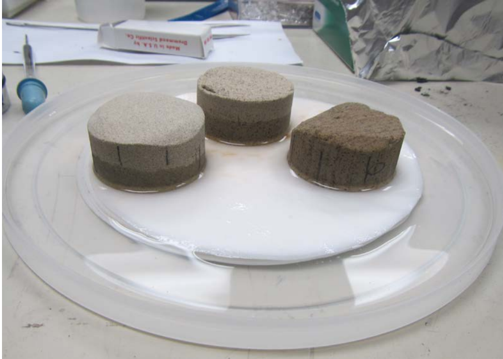
Fig. 4: Capillary Uptake: 10 min., Saturation of 1900 Stone
