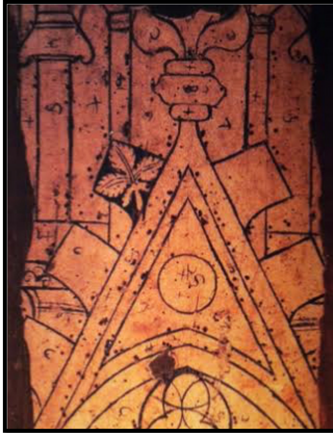
Figure 1. A medieval glazier's table used for design outlines for stained glass. Image from Sarah Brown, Stained Glass: An Illustrated History . 1992: 18.
