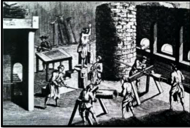
Figure 13. Cutting and flattening the muff glass. Image from Linda Cannon, "History of the Techniques and Materials." 1991: 54.
