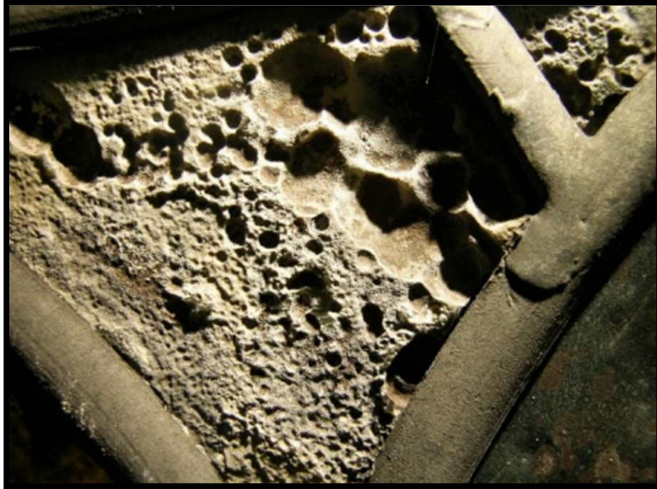
Figure 19. Glass pitting on a stained glass window from Caterbury Cathedral. Image from Leonie Seliger, “The South Oculus Window of Canterbury Cathedral.” 2011: 5.
