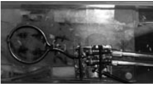
Figure 2. The rat is lying on his back in the MRI with his tail on the right. He is seen from the undersurface through a transparent plate. The four subcutaneous implants are located within the diameter of the 40 mm circular RF surface coil.
