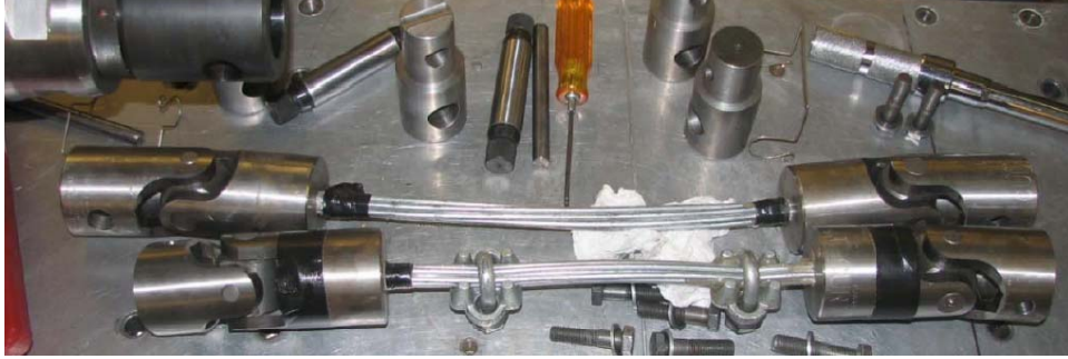
Figure 2.8: Experimental setup of the seven wire parallel strand. More images on the experimental setting are provided by Noyan et.al. [31].
