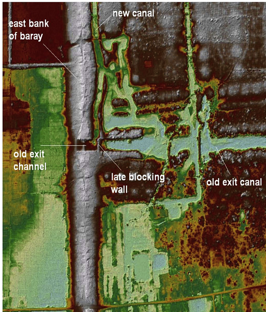
Fig. 10. LiDAR-derived image of the former eastern exit of the East Baray (shown as “F” on Fig. 5) and its conversion to an inlet fed by a new canal from the north, running down the outside of the eastern bank of the baray (Image courtesy of the Khmer Archaeology LiDAR Consortium).
