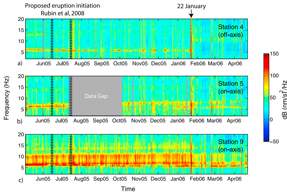
Figure 9. Average daily spectral signature for the three eruption surviving (deployment 3) stations: (a) station 4 off axis, (b) station 5 on axis, and (c) station 9 on axis. Each vertical slice represents the average spectral signal from one 24 h monitoring period, which is established using Welch’s method with 1 h nonoverlapping windows. Gray shaded areas represent gaps in data coverage. The large amplitude broadband signals observed on 22 January 2006 are unique to all four deployments and have been interpreted to represent brittle failure in response to dike intrusion [Tolstoy et al. , 2006]. Notably, there is no 6 Hz tremor immediately following the eruption at station 4.
