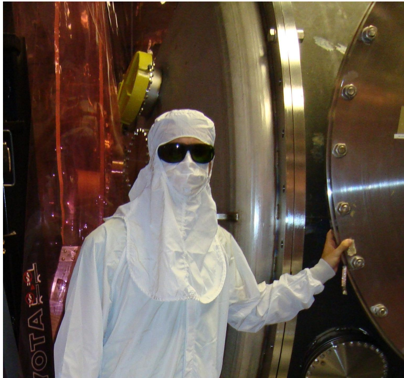
Figure 1-7: Protective equipment is required for activity close to the vacuum system in order to protect the the interferometer from contamination. The figure shows the Author participating in maintenance work at the LIGO Hanford observatory.
