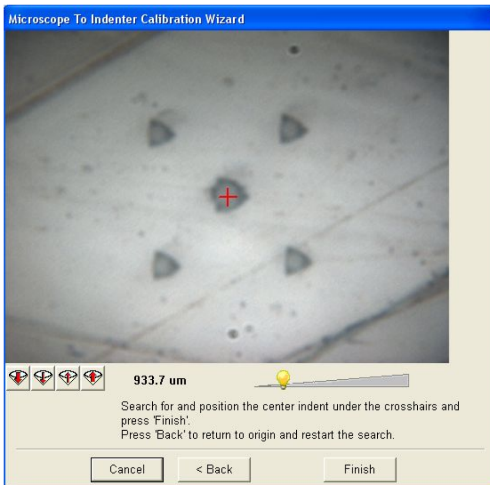
Figure 6.4: Microscope to indenter properly centered before clicking “Finish”.
