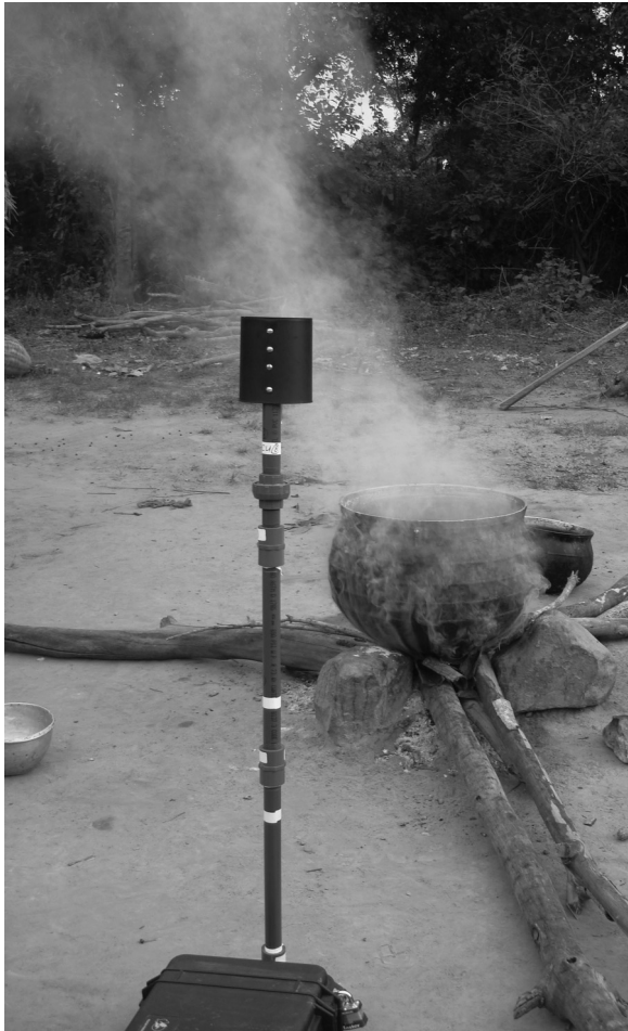
Photo 1. Area air sampling system in weatherproof case during 24-h monitoring period of an outdoor kitchen .
