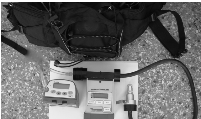
Photo 2. Personal air sampling system including Triplex cyclone, Personal Data Ram, battery operated TSI Sidepak SP530, and waist pack .
