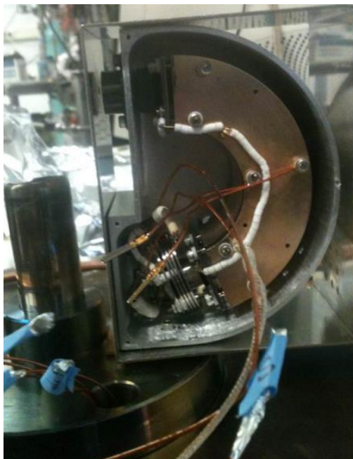
Figure 3.8 Photograph of electron energy analyzer with MCP for photoelectron detection
