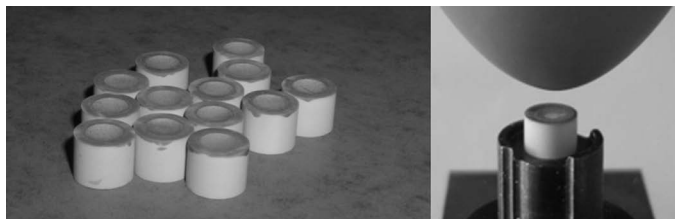
Fig. 2. (left) Porous ceramic cylindrical substrates used as backings, with spherically machined surface. (right) Structure during film deposition process by pad-printing. The silicone rubber pad (shown at top of image) is being lowered to deposit a layer of ceramic slurry on the curved surface of the substrate, upon which the rear electrode has previously been deposited.
