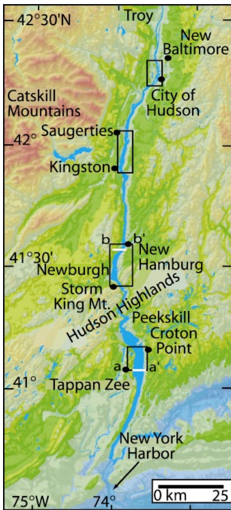
Figure 1. Hudson River estuary studied areas (boxes) surveyed with side-scan sonar, multibeam bathymetry, high-resolution CHIRP, and sediment cores (Bell et al., 2000). Bridge crossings (a-a', b-b') are shown in Figure 2.
