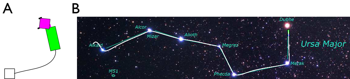
Figure 2. A) The lower-level controller directs the truck to a sub-target (white square). The black trace shows the path of the back of the truck. B) The lower-level controller directs the truck to trace the constellation Ursa Major (white line is the path of the truck) by approaching sub-targets at the locations of the stars. The sub-targets appear one at a time; when the back of the truck arrives close to the current sub-target, it is replaced by the next sub-target. Photo by Akira Fujii.
