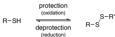
Figure 1.6. A protection/deprotection scheme for thiol: oxidation to the disulfide and reduction to the thiol.
