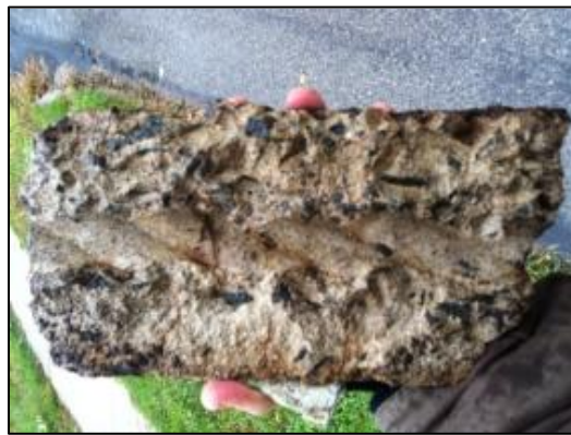
Figure 80: Sample from Battery Mahan 1 Lower, southern extension, showing an impression of a Ransome bar in the concrete
