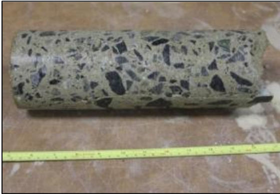
Figure 83: Battery Mahan 1 Upper Core (1898-1900), note the lift line
