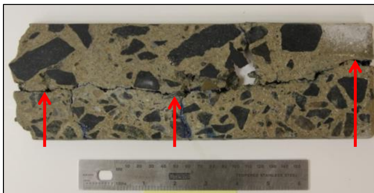
Figure 88: Section of the Mahan 1 Core (1898-1900), showing a large number of platy and crushed coarse aggregate
