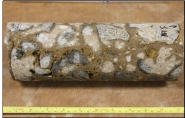
Figure 84: Battery Sumner 1 Upper Core (1891-1897), note the lift line
