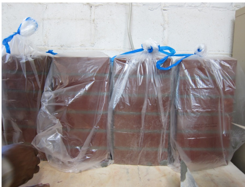
Figure 5 - Samples Curing in Sealed Plastic Bags for Initial 48 Hours
