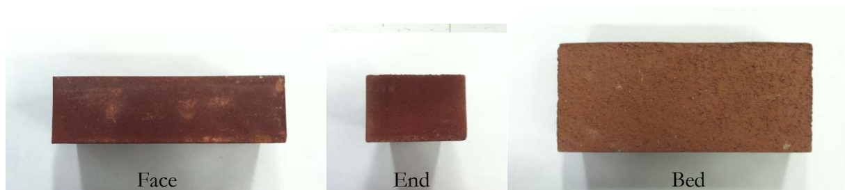
Figure 2 - Photos of standard Watson town Brick Used in Experiment
