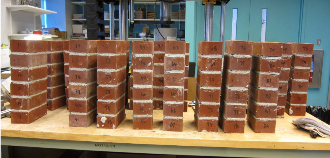
Figure 17 - 7-day Cured Sample Prisms Ready for Testing
