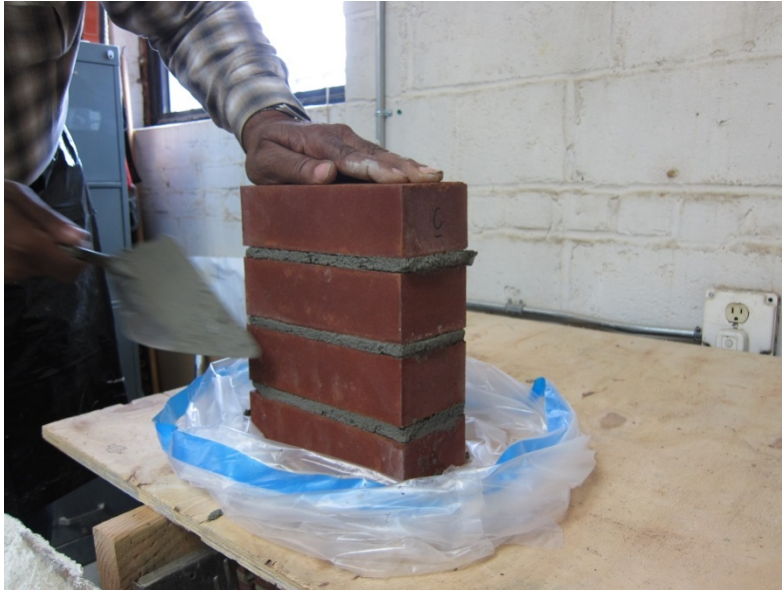
Figure 4 - Mason Constructing Sample Prisms
