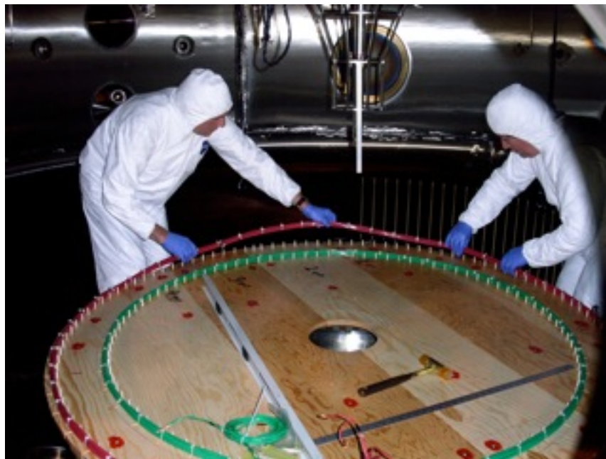
Figure 4.1: Rick Lations and Darren Garnier install the ‘copper plasma’ for calibrations. The 76 cm and 92 cm coils can be seen in green and red, respectively.
