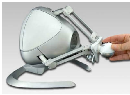
Figure 1: The Novint Falcon, a three-dimensional force feedback joystick.
