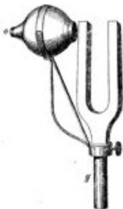
Fig. 3.3. August Lucae’s rudimentary masking tool used in therapy for patients suffering from subjective noises. The device consisted in a resonator to be placed in the ear and a tuning fork selected on the basis of the subjective noise’s acoustic properties. “A high subjective hissing sound ( ein hohes subjectives Zischen ),” for example, was treated with a tuning fork set to low C. The objective tone from the tuning fork was initially played for patients for two minutes but this was extended to as long as 10 minutes, with the volume also increasing gradually over the course of a session. From: August Lucae, Zur Entstehung und Behandlung der subjectiven Gehörsempfindungen (Berlin: Otto Enslin, 1884), p. 39.
