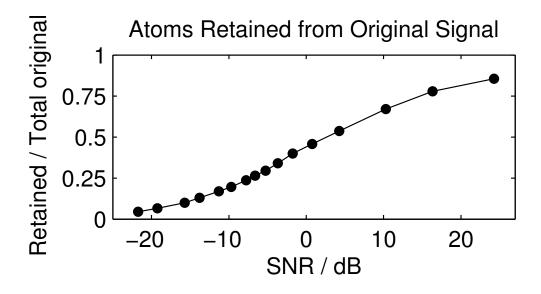
Figure 3.3: Percent of MP atoms retained from the original signal as the noise increases.
