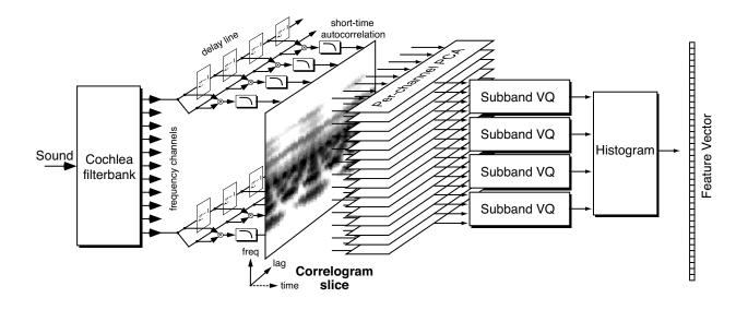
Figure 7.5: Block diagram of the calculation of the subband autocorrelation PCA feature vectors.
