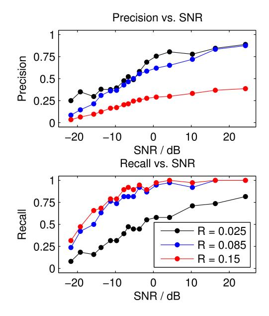
Figure 3.4: Detection, precision, and recall vs. SNR at three LSH radii.
