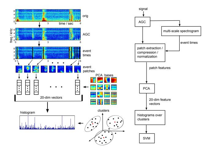
Figure 5.1: Block diagram of transient feature system, with examples of data.
