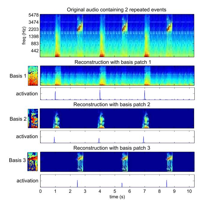
Figure 6.1: Convolutive NMF decomposition example showing three basis patches and their corresponding activations, as learned from a piece of toy data.
