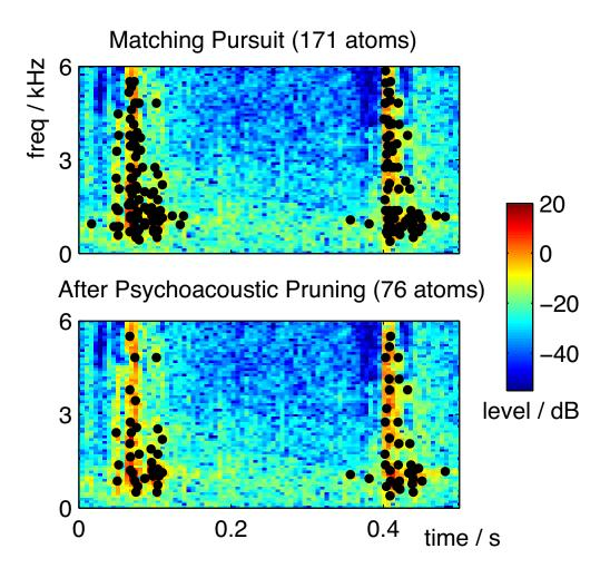
Figure 3.1: Matching pursuit atoms used to represent audio events, shown as dots at the centers in time-frequency overlaid on the spectrogram, before and after psychoacoustic pruning.
