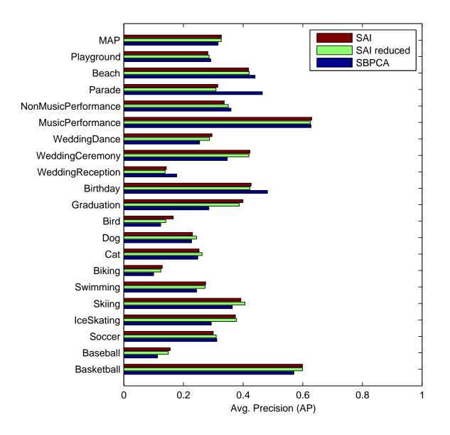
Figure 7.4: Comparison of SVM systems using: full set of 24 SAI rectangles (24,000 dimensions), a reduced set of 8 SAI rectangles (8,000 dimensions), and the simpler SBPCA features (4,000 dimensions).
