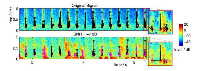
Figure 3.5: Original query patterns (top), and mixture detection results (bottom). Black pairs are correct detects; magenta are false positives.
