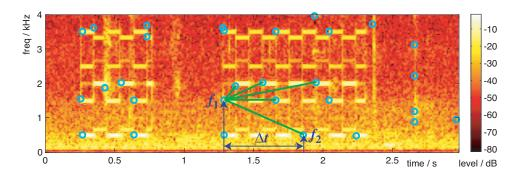
Figure 3.2: Example formation of atom pairs for hashing, defined by the triplet of  $(f_1, f_2, \text{and } \Delta T)$ .
