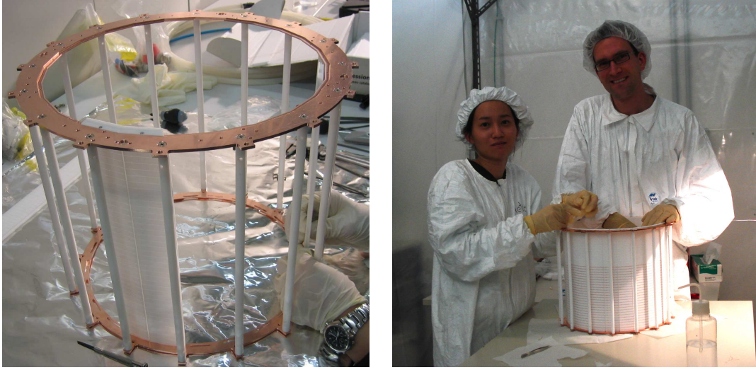
Figure 3.3: Picture of the top and bottom copper ring frames of the TPC, along with 16 PTFE support rods and two interlocking PTFE panels during panel installation (left), and a picture of the TPC during the fabrication of the field shaping copper wires (right). From left to right: the author and M. Schumann (Rice University).
