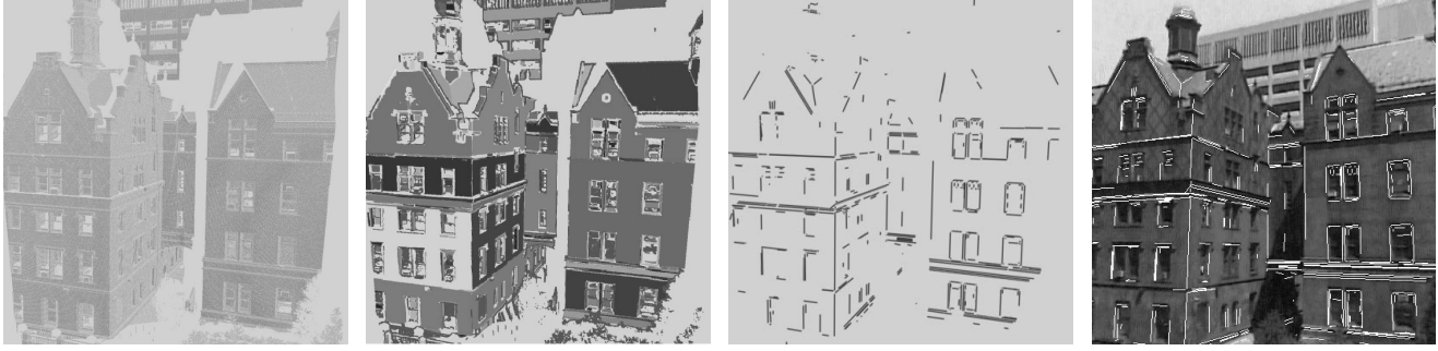
Figure 2: a) Range data scan, b) Planar Segmentation (different planes correspond to different colors), c) Extracted 3D lines generated from the intersection of planar regions, d) 3-D lines projected on the image after registration.
