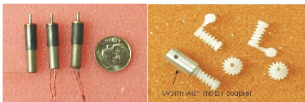
Fig. 12. Left: Smoovy motor with magnetic wire, Right: Worm gear
