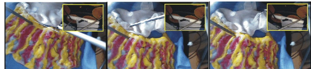
Fig. 4. The device was used in a suturing experiment within a laparoscopic training box. The image provided by the device was sufficiently clear to perform the task without using any additional image sources. The surgeon's assistant was able to adjust the view at the surgeon's request by joystick control of the camera's pan, tilt and translation axes.
