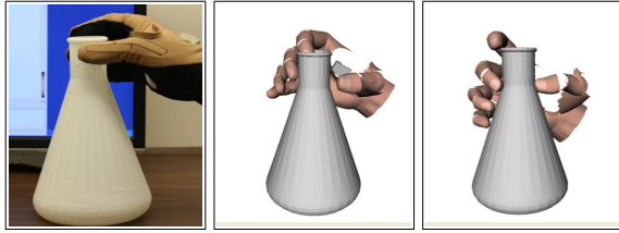
Fig. 4. Grasp planning using human data. Left: grasp executed by human operator. Middle: Low-dimensional approximation of human grasp, also affected by measurement noise. This posture, which only approximates a correct grasp, is used as input for the grasp planner. Right: form-closure grasp found by the planner based on the input data.
