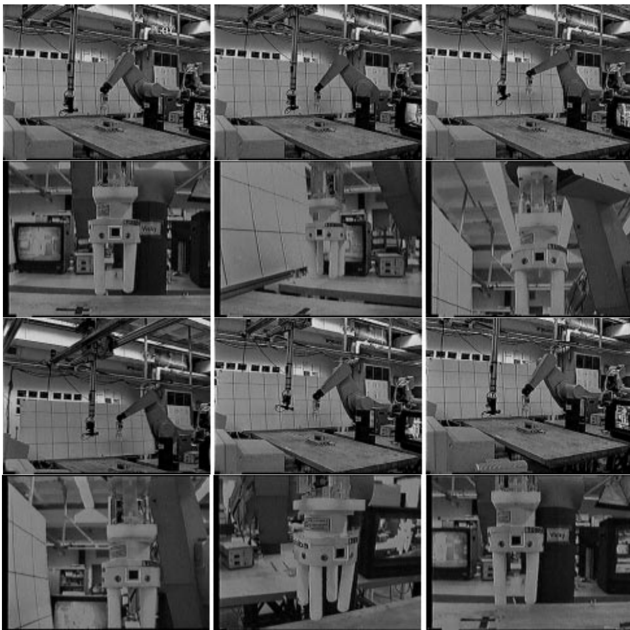
Fig. 22. Six sequential snapshots while regulating camera-to-hand distance. Rows 1 and 3 are image stills from a video camera and Rows 2 and 4 are image stills from the robot camera. Top left to bottom right: (top left) from home the hand moves diagonally away from and to the left of the camera and results in camera pan and side translation X . The hand moves up and results in a camera tilt and upward translation Z . The hand then moves both downward and toward the camera, returning to its home position (bottom right). The final camera position has the target centered and parallel to its image plane, with the desired camera-to-target distance.
