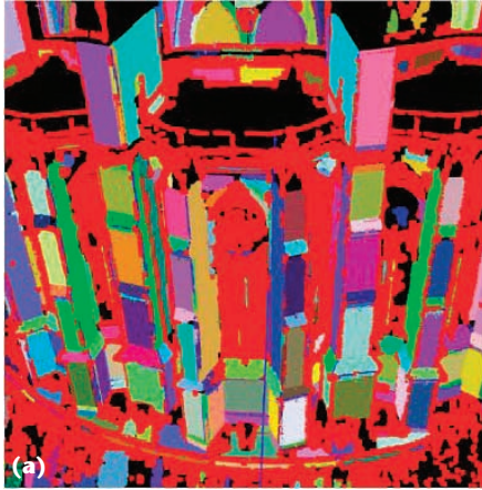
2 (a) Segmentation detail in a scan of the cathedral data set. Different colors represent different planes. The red color corresponds to the unsegmented (nonplanar) parts of the scene. (b) Registration of lines between a pair of overlapping scans of the cathedral: left lines (white), right lines (blue), and matched lines (red and green). Due to the overlap of the matched lines, sometimes only the red or the green component dominates.
