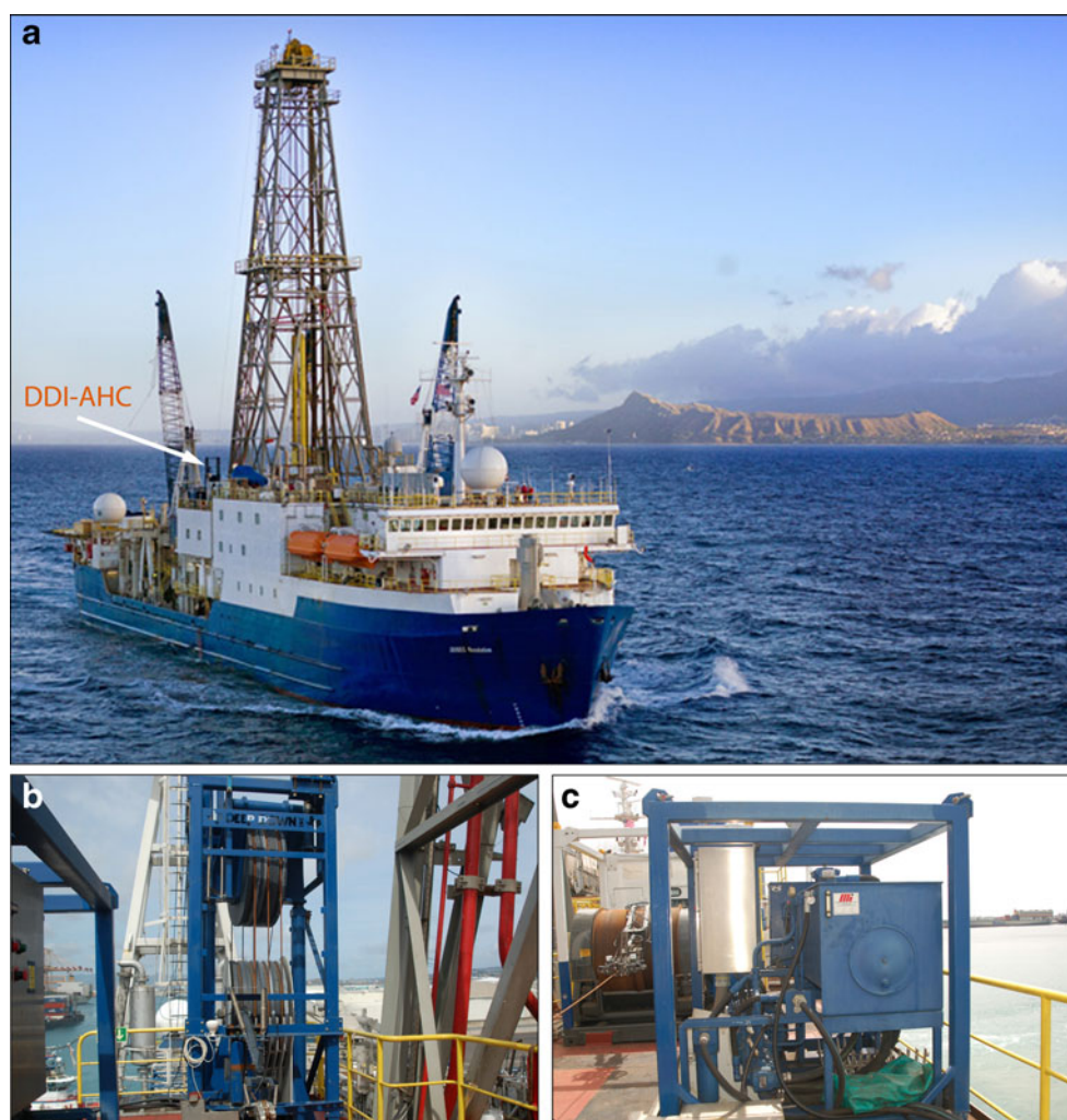
Fig. 1 a The JOIDES Resolution deep-sea research-drilling vessel showing the location of the heave compensating system (photo courtesy of USIO-IODP). b Sheave components of the DDI-AHC wire-line heave compensator. c The hydraulic power unit and winch
