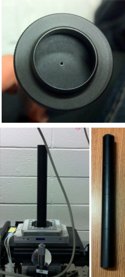
Figure 2-15. Alignment tool for coarse alignment of the system. The alignment tool is ~20 inches in length. Small diameter pinholes are placed at either ends of the pinhole. It is placed in place of the objective lens and the lasers are allowed to pass through the two pinholes to confirm optimal alignment.
