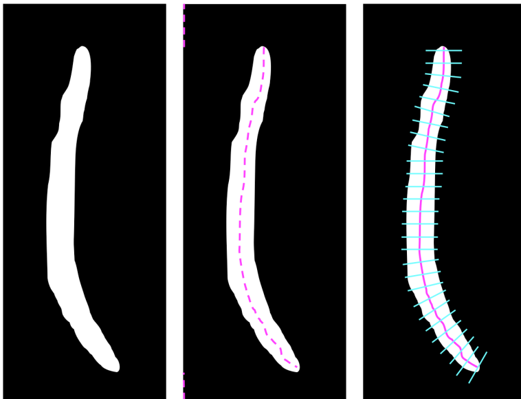
Figure 5-3. Sketch representing details of the development of image processing module that enabled extraction of morphometric features of primary cilia. (A) Extraction of primary cilia from the large scan area, cleaning and thresholding to enhance contrast (B) Determination of highest intensity pixel across each scan line. Highest intensity pixels
