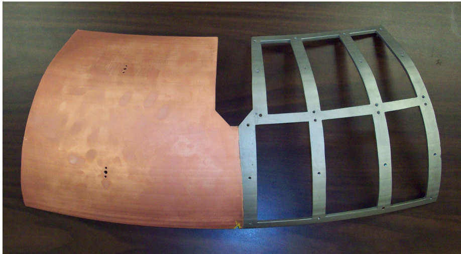
Figure 2.2: Picture of an HBT-EP wall segment after copper plating, but before chrome plating. This shell has a large cutout at the top center for an interferometer beam.
