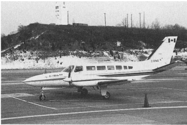
FIG. 2. INTERA KENTING's Cessna 404 configured for airborne gravity surveys.
