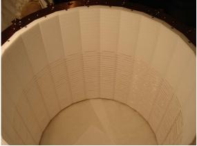
Figure 3.18: Picture of the top and bottom copper ring frames of the TPC, along with its 16 PTFE support rods, during the installation of the PTFE panels (left), and a picture of the TPC during the installation of the field shaping copper wires (right). Each panel is inserted in a slot in the bottom copper ring and screwed to the top copper ring.
