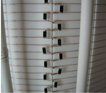
Figure 3.30: Picture of the resistor chain of the field shaping wires voltage divider circuit after the modification underground (left). A closer view of the modified solder points of the resistors to the field shaping copper wires (right).
