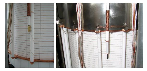
Figure 3.24: Pictures of the cathode (left) and anode (right) feedthrough connections. The connection of both feedthroughs are made below the LXe level with their copper braids reaching below the LXe. The connections are made with bare copper wires. The cable bundles from the bottom and bottom veto PMT arrays are also visible.
