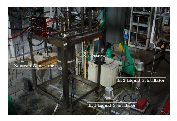
Figure 5.25: Experimental setup for the  $\mathcal{L}_{\text{eff}}$  measurement at 3 keV (23°). For this angle both EJ301 neutron detectors are in the horizontal plane of the neutron generator and the LXe detector.
