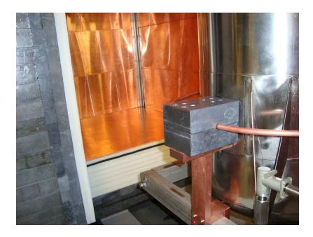
Figure 3.40: Picture of inner cavity of the XENON100 passive shield. A copper support holds the lead brick arrangement used to attenuate high energy  $\gamma$  rays from the AmBe neutron source used for calibration. Also visible in the lower right corner is a mount of the cryostat and the mechanical coupling (Sec. 3.2.2) that allows the leveling (Sec. 4.2.3) of the cryostat from outside the passive shield.
