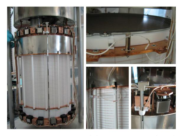
Figure 3.29: Picture of the long level meter (left), one of the short level meters (top right), and two of the temperature sensors (bottom right) installed during the first opening of the XENON100 cryostat after its original installation.
