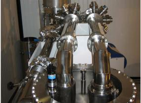
Figure 3.17: A top view of the cryostat lid (left) and of the entire top assembly and cooling tower connection (right). The LXe level adjustment motion feedthrough is visible on the left along with the two flanges for the future anode and cathode high-voltage feedthroughs. The white wooden support represents the position of the passive shield door underground.
