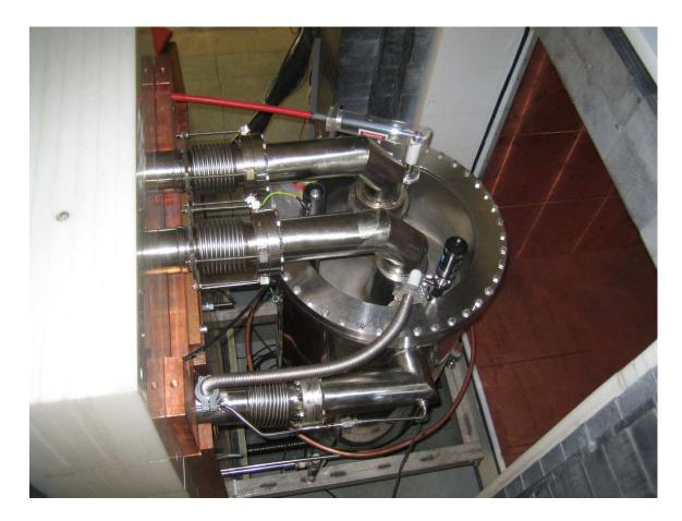
Figure 3.27: The XENON100 detector inside the passive shield with anode, cathode, and vacuum connections completed. The circular copper tube can be used to irradiate the detector at various azimuthal positions when the shield door is closed.
