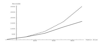
Figure 11: Indexing effect in taking the whole transitive closure
