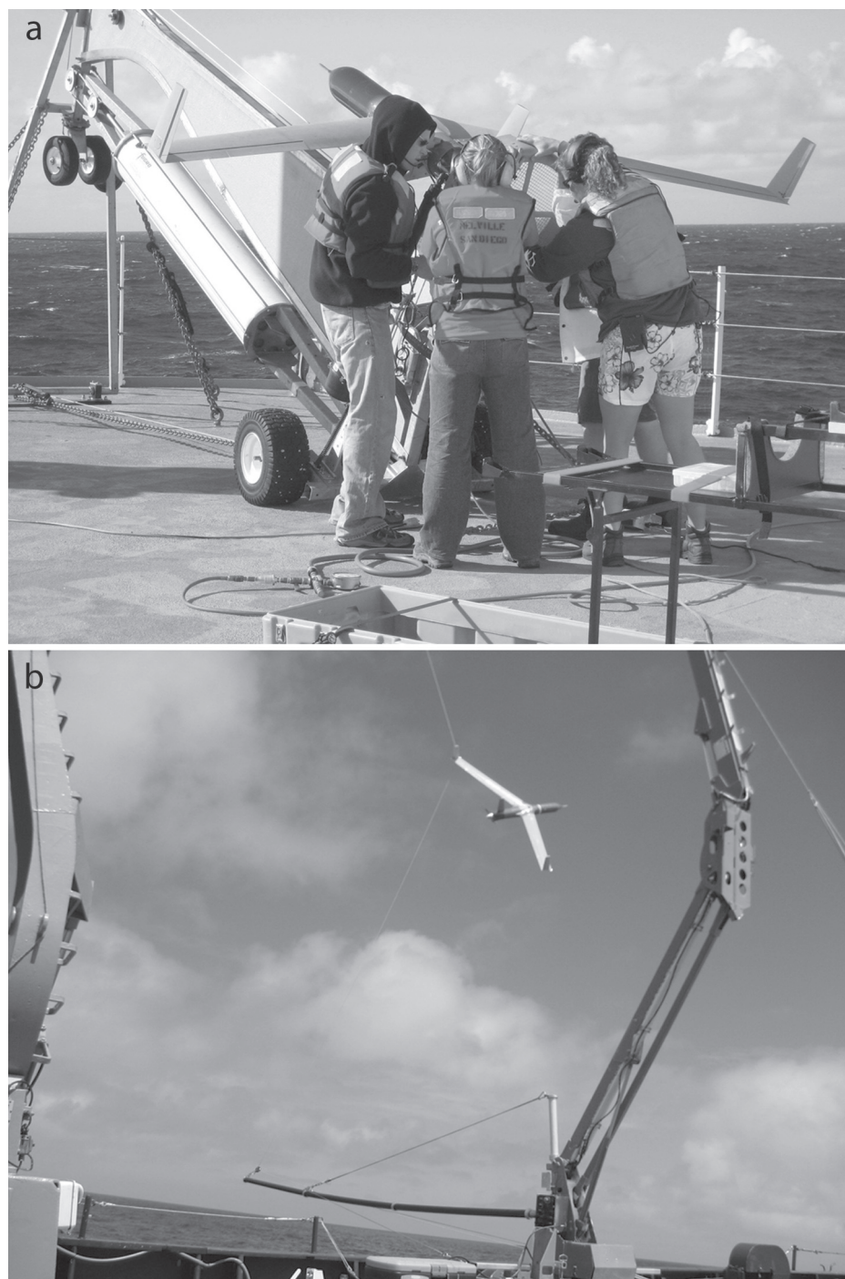
Fig. 1. GeoRanger unmanned airborne vehicle (a) on catapult in preparation for launch and (b) just after capture. Original color image appears at the back of this volume.
