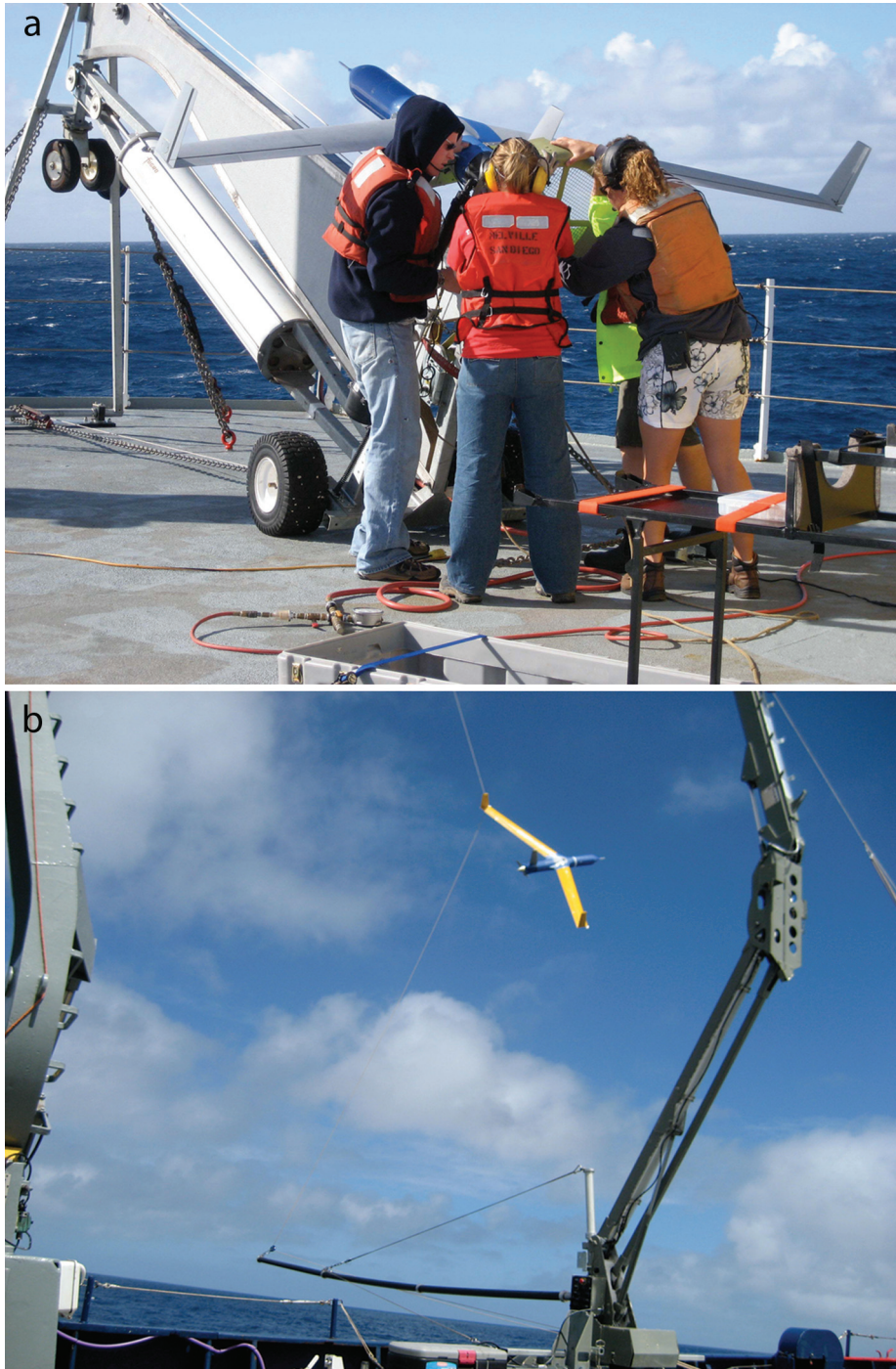
Fig. 1. GeoRanger unmanned airborne vehicle (a) on catapult in preparation for launch and (b) just after capture.
