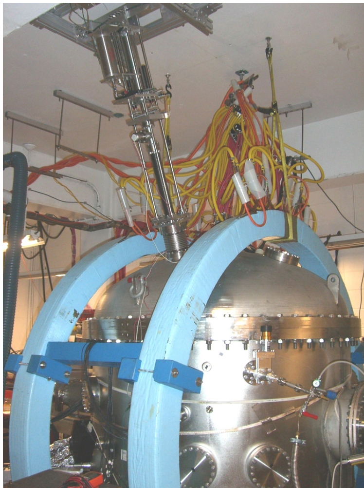
Figure 4.1: This photograph shows the retractable emitter installed on CNT. It is attached to the ceiling and connects to the vacuum chamber via a flexible bellows that allows for position adjustments.
