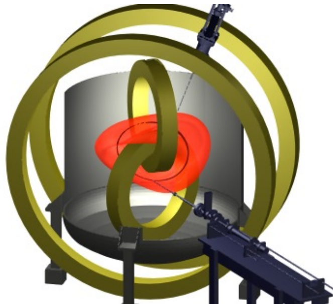
Figure 2.2: A drawing of CNT illustrates the confining volume in red, four planar coils in gold, and two filaments held on the magnetic axis by ceramic rods. The four probe array is represented on the bottom while the retractable emitter inserts from the top.
