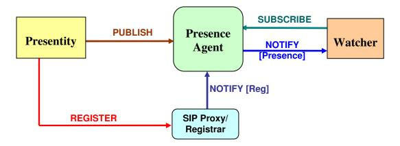
Figure 1 Basic block diagram of a presence system
