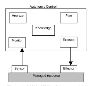
Figure 1: IBM MAPE-K reference model.
