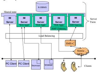
Figure 3: The IM service architecture.
