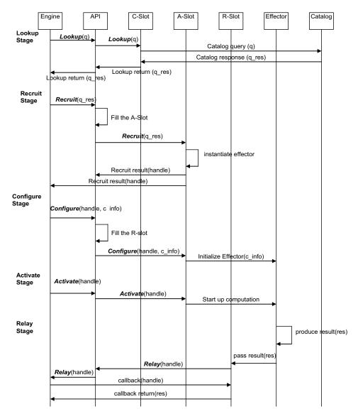
Figure 6: The various stages of effector execution.
