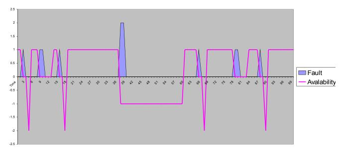
We notice the dip in availability in the center of the graph due to manual repair of the disk failure.
