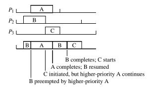
Figure 7: The behavior of an RTOS with fixed-priority preemptive scheduling. Rate-monotonic analysis gives process  $P_1$  the highest priority since it has the shortest period;  $P_3$  has the lowest. A would have missed its deadline (the tick mark) had it not preempted B.
