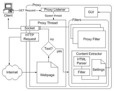
Figure 13. Architectural diagram of the system
