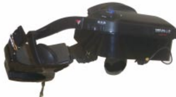
Figure 11: The Remote Reality HMD. The small lapel microphone attached to it for the audio sub-system can be seen in sitting in the middle of the front visor panel.
