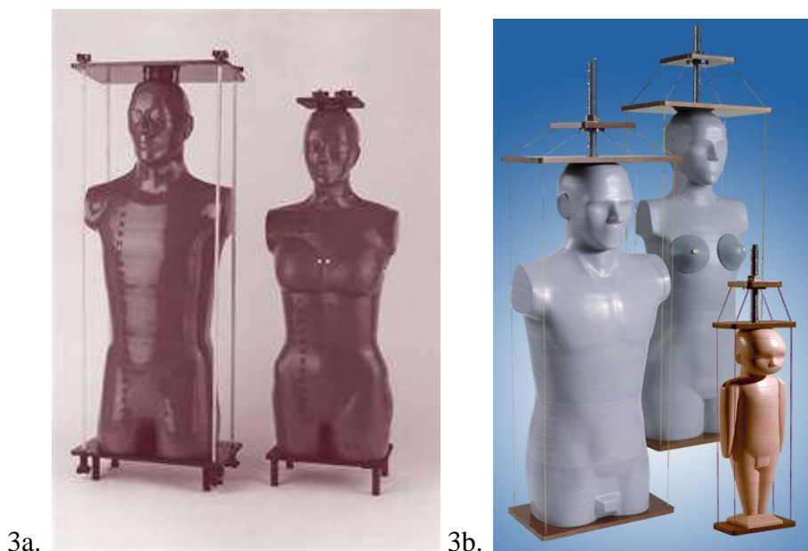
Figure 3. a) Rando-Alderson dosimetry verification phantom. b) CIRS dosimetry verification phantom.
