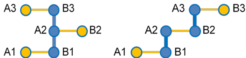
Figure 1.12 Tight-binding diagrams from ABA (left) and ABC (right) trilayer graphene. The yellow and blue lines represent intra- and inter-layer nearest-neighbor coupling. At the K point, the intralayer coupling becomes zero. The atoms in yellow then become non-bonding monomers and the atoms in blue form a trimer in ABA trilayer and two dimers in ABC trilayer.
