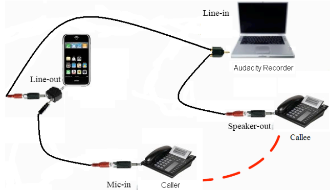
Figure 5: Setup for measuring hard phone latency
