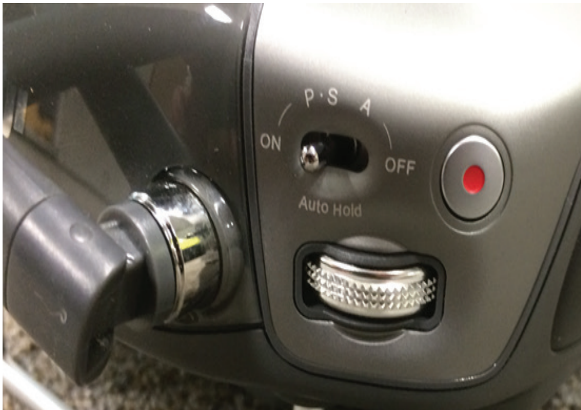
Figure 8. Transmitter with flight mode P, S and A
