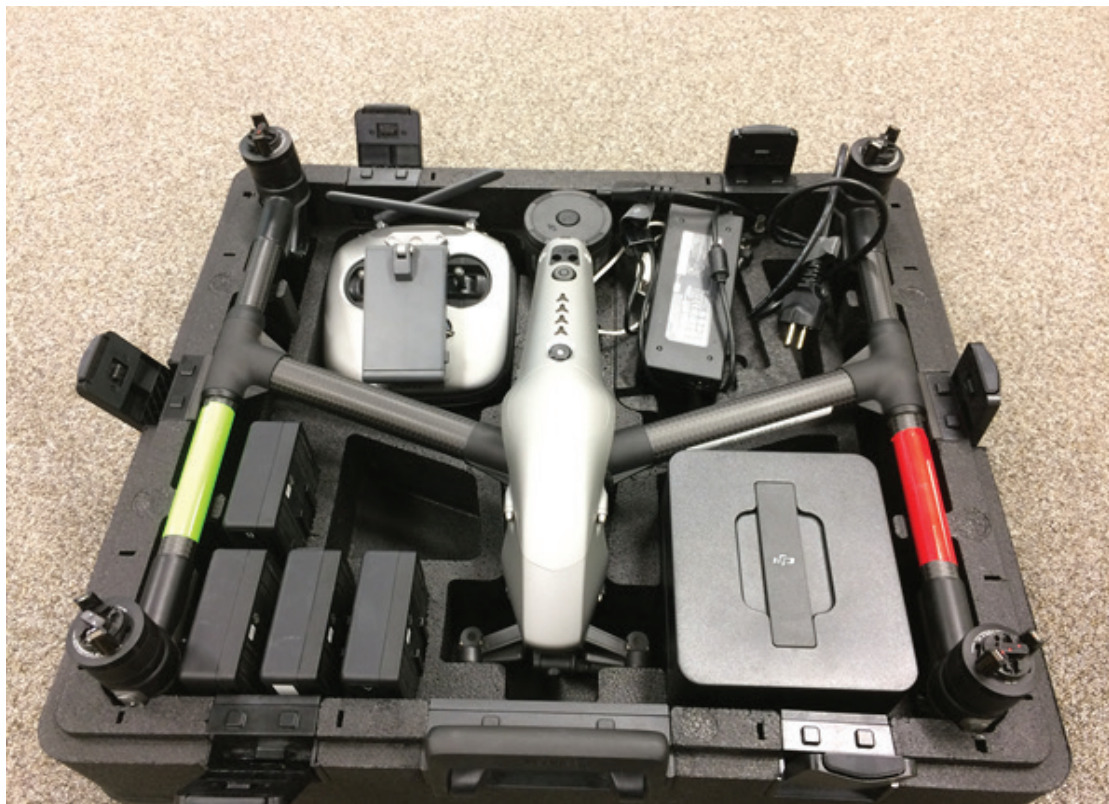
Figure 7. A professional-level drone (DJI Naza Inspire 2). On the right side is a 4K camera in the box. On the left side are batteries and the remote control (transmitter) unit. This quadcopter can lift its landing gears up and it may fly over 20 minutes. It is also possible to control the camera and drone with smart devices like tablets or smartphones.
