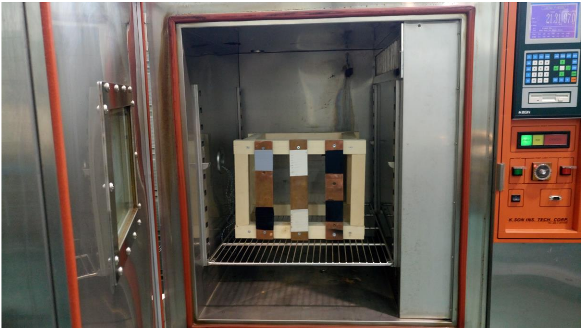
Figure 10 - The bus bar rig inside the oven
