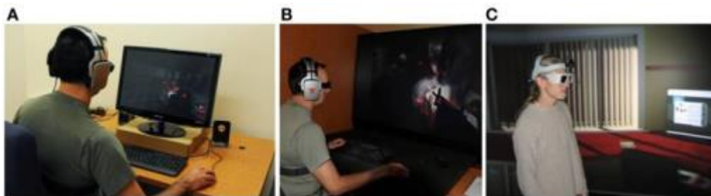
Kuva 4. Examples of immersion levels: (A) a non-immersive VR system, (B) a semi-immersive VR system, and (C) an immersive VR system (Baus, Bouchart 2017)
