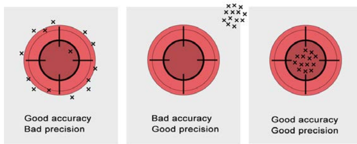
FIGURE 7. Accuracy vs. precision.
