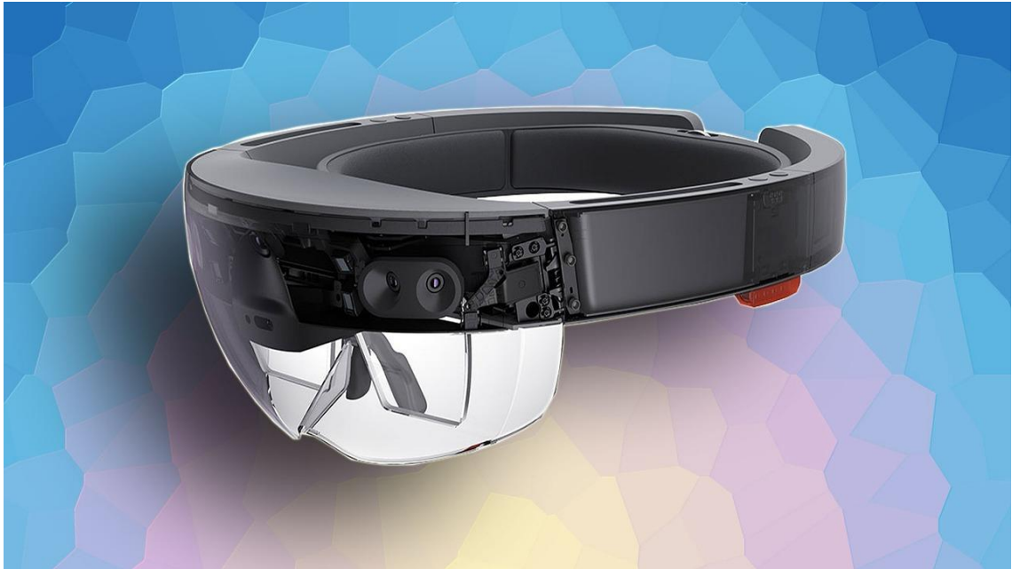
Picture 1 Microsoft HoloLens MR glasses have integrated speakers and sensors observing the environment and user's actions. Picture used under CC0 Creative Commons licence.
