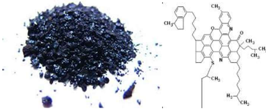
Figure 1. Solid asphaltene (left) and the hypothetical chemical composition of asphaltene (right). [8] [3]
