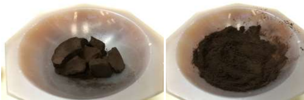
Figure 20. The dried samples were easy to drop from the bottom of the used plastic bottle to a mortar. The sample broke from bigger pieces (left picture) to fine dusty dry powder (right picture) with just lightly pressing with a plastic spoon.
