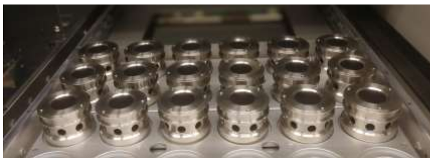
Figure 27. The calibration samples ready to be measured in the auto sampler of the instrument (blank and 8 calibration samples with their duplicates).
