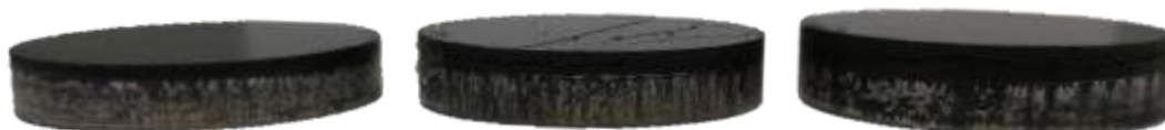
Figure 18. 3, 4 and 5g of blank sample on top of 10ml of Boreox in aluminium cup pressed with 100kN.
